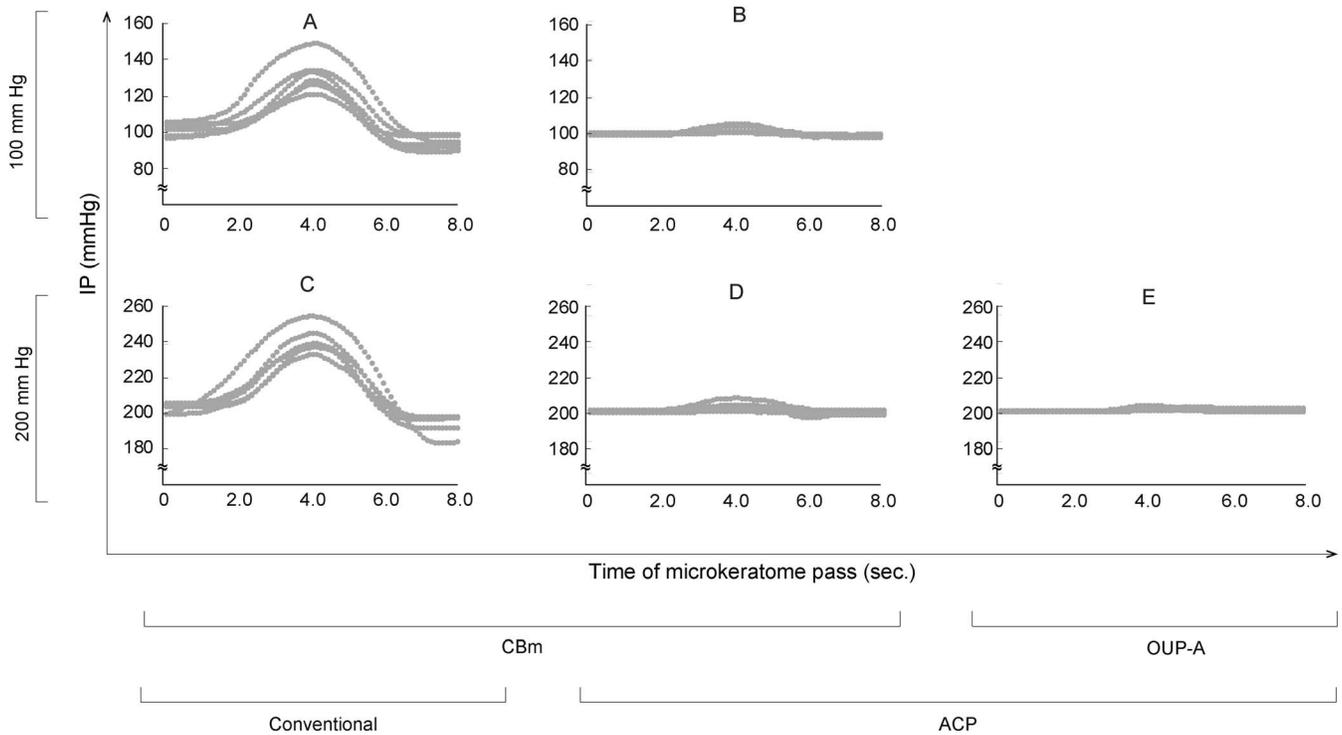
**Figure 1.** Changes in artificial anterior chamber IP at microkeratome passing. The IP change during dissection was measured every 1/10 second by a real-time pressure sensor connected to the infusion line. While the groups in which ACP was used (groups B, D, and E) showed constant IPs, the conventional groups (groups A and C) had elevated IPs during the microkeratome pass.
